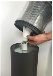
11.) When the lamp is secured in the socket, gently slide the bollard head back down to the housing. Be sure to line up the metal tabs on the bollard head housing plate to the hex screw holes in the housing.
