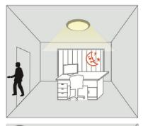
If there is no more movement, the light dims to stand-by dimming level after hold-time.
