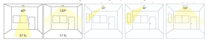
This shows how optics change the number of footcandles on the floor. It also shows how optics affect light distribution. You needed specialized optics to achieve the fc and Max/Min ratio presented in this photometric study.
