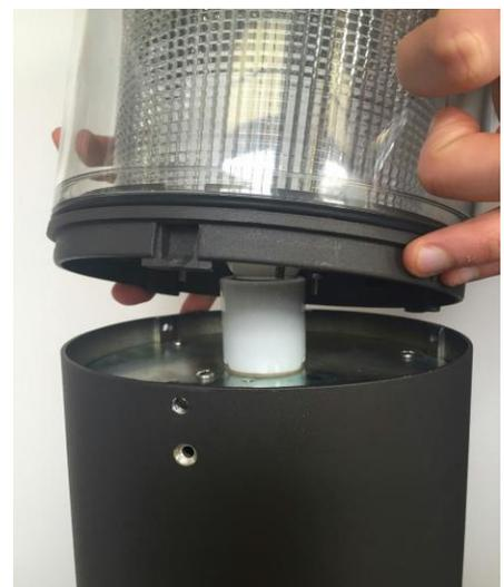
12.) With your fingers and an Allen wrench, screw in the three hex screws so they are flush with the bollard housing. Make sure the hollowed-out end of each screw faces away from the bollard.
